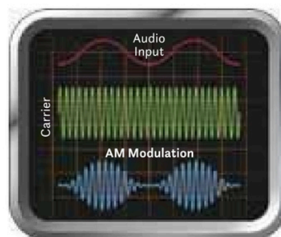
In AM modulation, the carrier frequency remains constant, and the signal amplitude changes.
