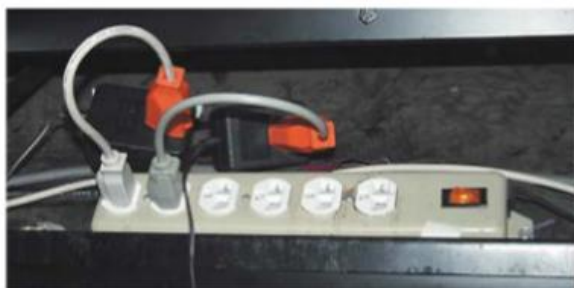
Figure 2: A couple of pigtails plugged into a power cord, with the pesky wall warts conveniently off to one side.
