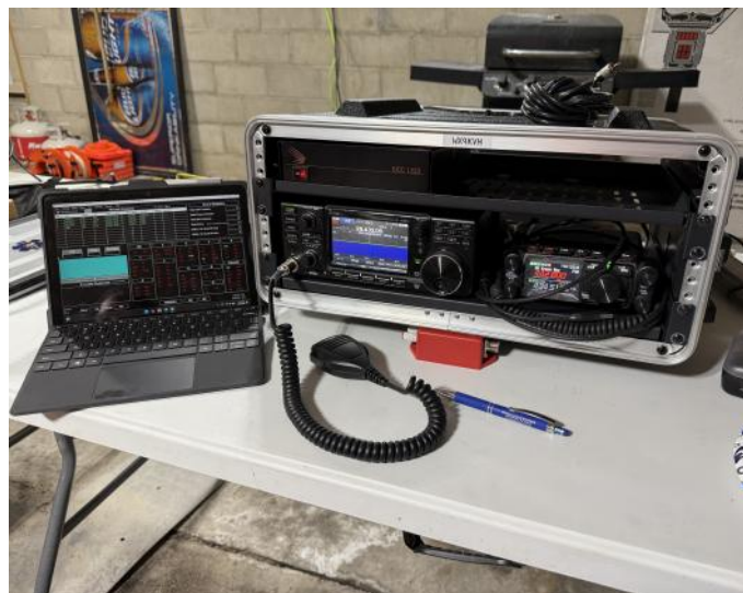
Kyle Van Hoogen (WX9KVH) also attended Field Day in Calumet County. Kyle is operating his portable station which contains an IC-7300, Yeasu FTM 500D, Samlex Power Supply, and a laptop running the N3FJP contesting software.
