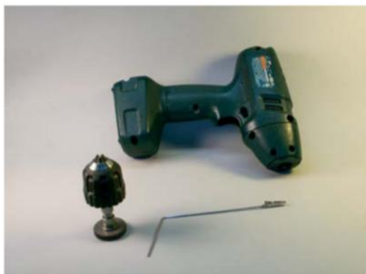
Before discarding a worn-out drill, remove the chuck and turn it into a handy "third hand."
