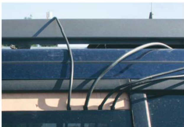
A small piece of wood or rigid insulation is easily shaped and notched to make a feed-line pass-through for your mobile installation.
