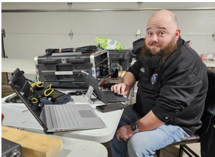
Kyle Van Hoogen (WX9KVH) also attended Field Day in Calumet County. Kyle is operating his portable station which contains an IC-7300, Yeasu FTM 500D, Samlex Power Supply, and a laptop running the N3FJP contesting software.
