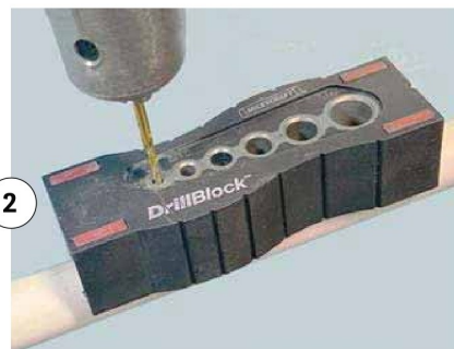
Using a center-drilling guide to accurately drill 1/8-inch guide holes through to both sides of the marked cross-arm positions on the vertical mast section.
