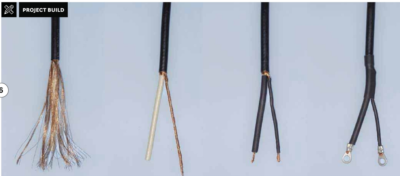
Sequence for separating the shield and center conductor into two separate conductors at the feed-point end of the coax pigtail.
