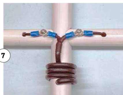
Forming the choke balun.
